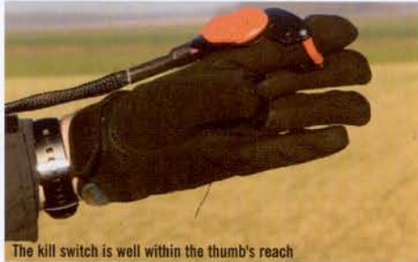
The kill switch is well within the thumb's reach
